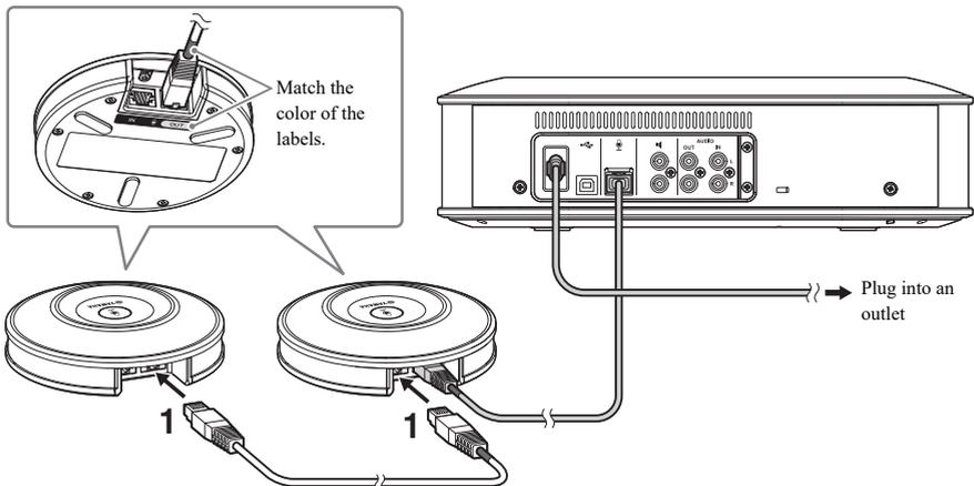
**1** Connect the second microphone to the first microphone.
