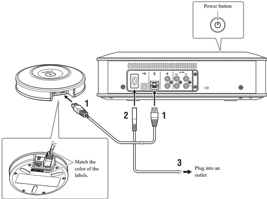
**1 Connect the microphone to the Control Unit using the microphone cable supplied with the product.**
